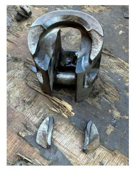
Potentially even broken pieces on the edges of the lift cradle (see photo on left).
