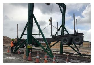
It is recommended to stand at the rear of the trailer, controlling the lift.
