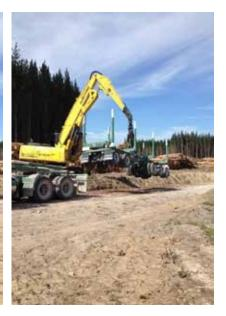
Driver ensures loader grabs trailer correctly and all chains are disconnected, signals OK and moves to safe area in view of loader operator before loader starts lifting.
