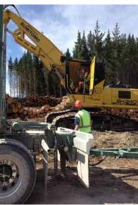
Truck driver connects trailer attachments while loader operator parks with cab facing driver and grapple lowered. Truck driver and loader operator discuss final loading details including where to place the logs on the truck and trailer. Driver moves into the agreed safe zone which could be the cab.
