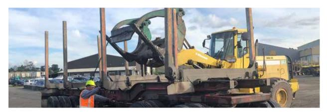
Complete re-positoning locking drawbar under trailer. The driver should not be under the trailer at anytime while it is suspended above ground.
