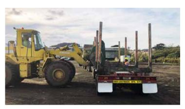
On the opposite side from the loader lift the chains onto the forks or use pogo stick if available.
