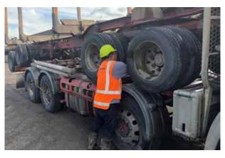
9 Secure trailer tie down chains securing trailer on truck.
