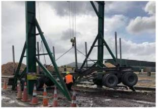
Lift trailer using lifting chain, only lift trailer high enough to spin draw bar. The front wheels of the trailer must be kept as close to the ground as possible. All practical steps should be taken to avoid being under the trailer, especially the head and torso.
