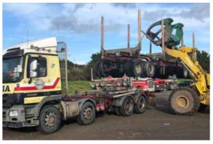
Reverse truck under trailer and lower trailer onto truck.
