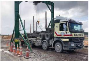
Reverse truck under trailer and lower trailer onto truck.
