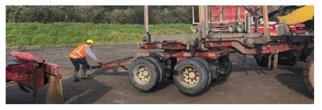
Turn draw bar keeping the trailer as close to the ground as practical whilst allowing the operator to maintain optimum control of the draw bar while re-positoning.
