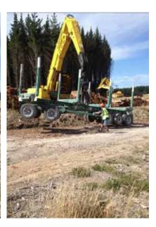
Loader moves to better position to lift trailer and gain a better view of truck driver as they come in to unhook the drawbar. Loader lifts trailer until front axle is off ground and rear axle is touching the ground making the trailer stable. Drawbar is at chest height, the optimal ergonomic position for the driver.
