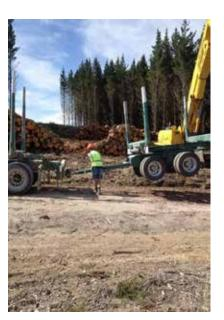
Driver stops and makes visual contact with loader operator. When visual OK is given the loader starts to slowly slew the drawbar towards the ring feder. Loader driver moves drawbar toward ringfeder with the truck driver guiding the tow eye. Truck driver always faces the loader operator and holds drawbar back from tow eye.
