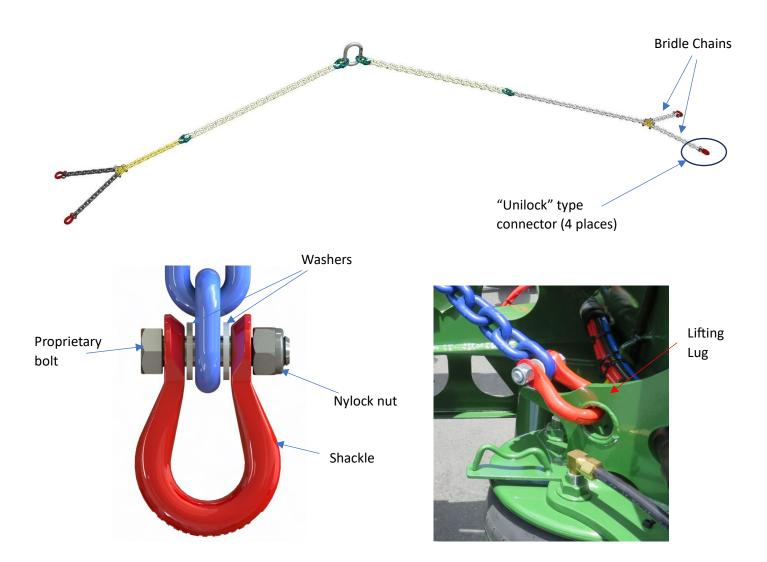
Warning! Failure of the connector during lifting may result in possible dropping of the trailer from height with risk of injury and/or equipment damage.
