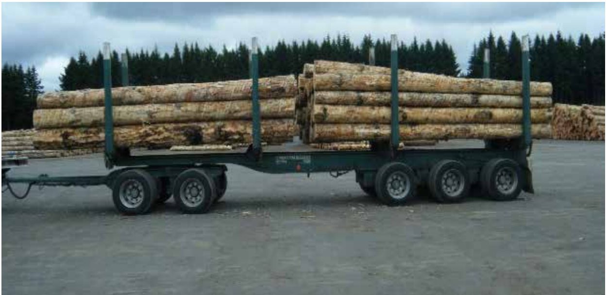
Preferred – Same load double bunked. Also note taper in the load.
