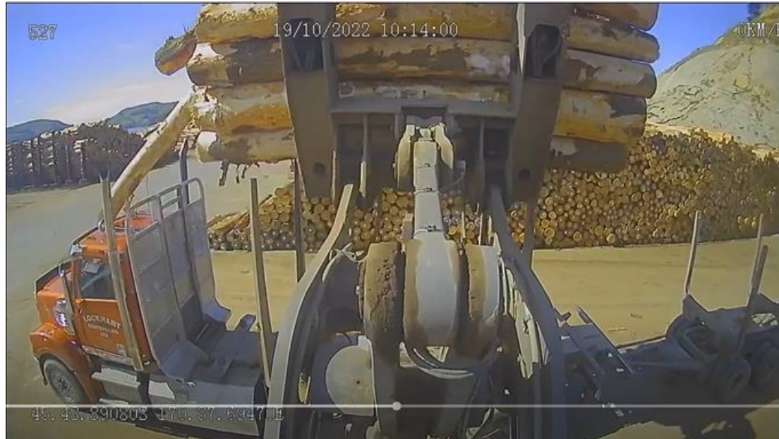
Figure 1. Example of log impacting truck cab roof.
