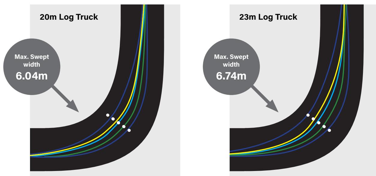
**The 23m vehicle needs 700mm more road width than a 20m vehicle to do a sharp 90° turn!**
