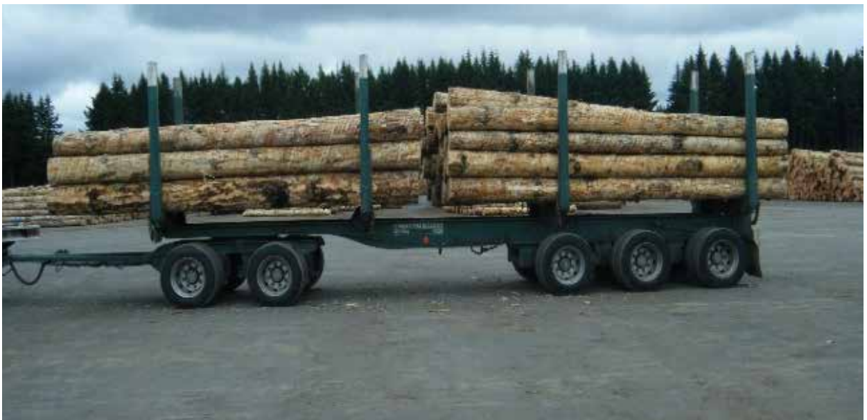
Preferred – Same load double bunked. Also note taper in the load.
