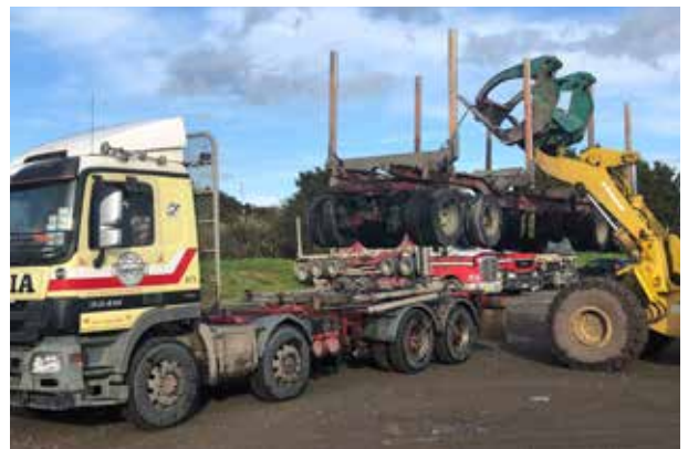
7 Reverse truck under trailer and lower trailer onto truck.
