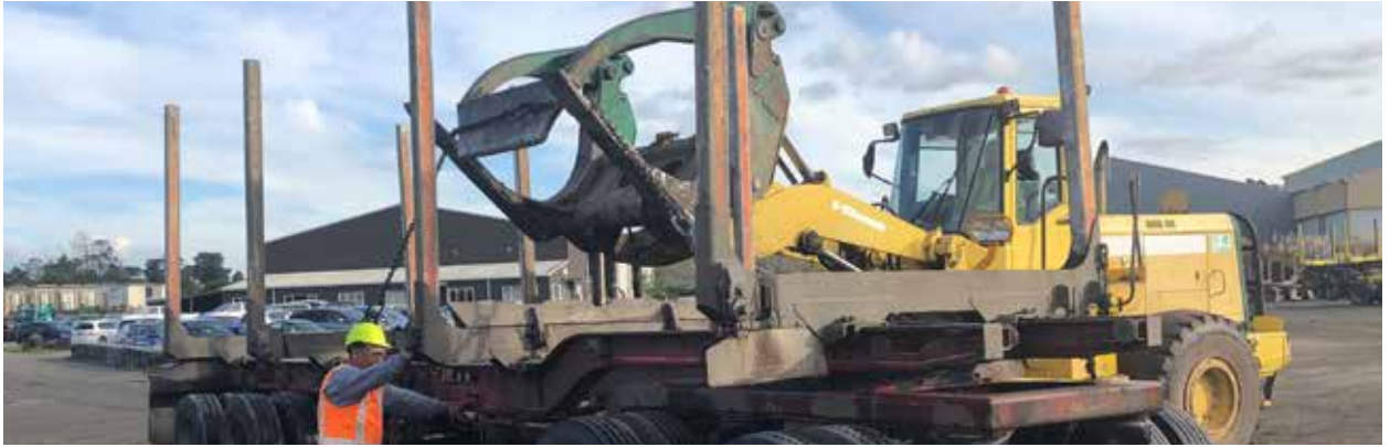
5 Complete re-positioning locking drawbar under trailer. The driver should not be under the trailer at anytime while it is suspended above ground.
