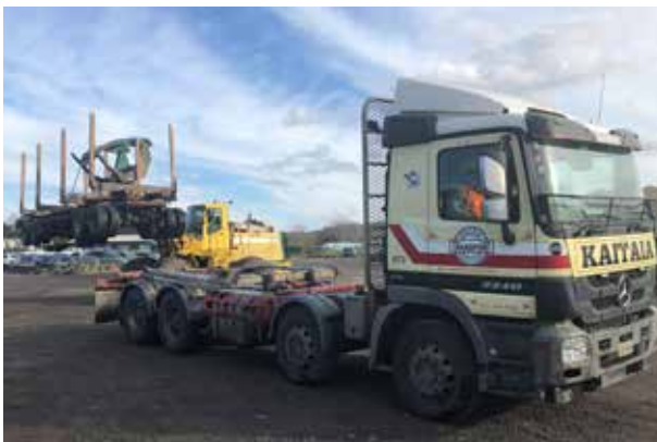
6 Once driver is clear the loader can lift the trailer.
