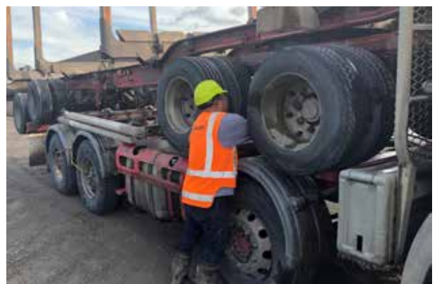
9 Secure trailer tie down chains securing trailer on truck.
