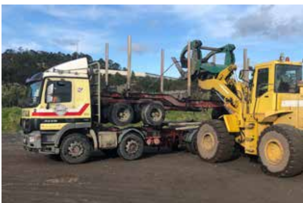
8 Position trailer on truck.
