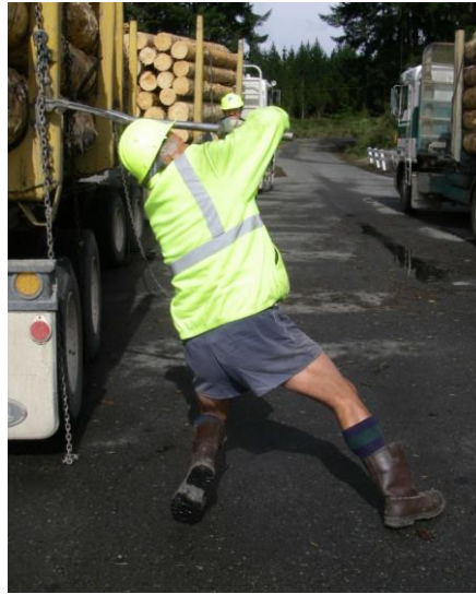
Figure 12. Chain tensioning, applying force
