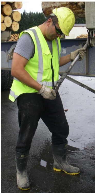
Figure 13. Chain tensioning using winch
